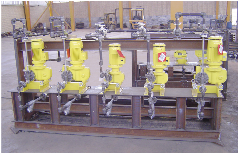
98% Sulfuric Acid Dosing Pumps for neutralization Package of Tabriz Refinery Project
